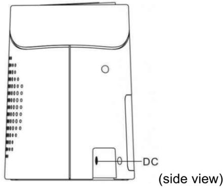
2. Plug the AC adapter into the port located on the back side of the unit marked "DC" and plug it into a standard wall outlet. As soon as the unit is plugged in it will turn on. To turn the unit off press the ON/OFF button on the remote or on the top of the unit.
